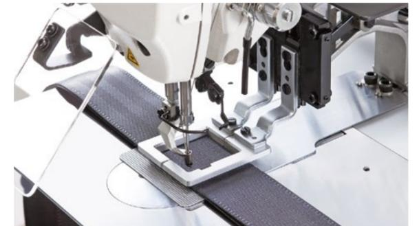
Example application: Reinforcing the stitching of seatbelts
