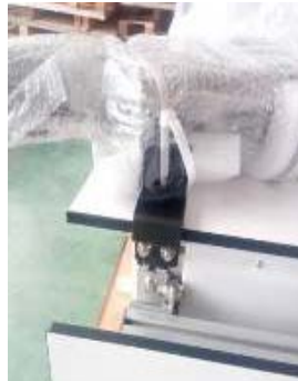
Cut the cable clip band to detach the sewing machine parts.
