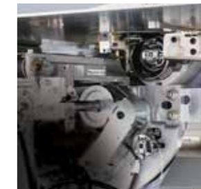
Automatic bobbin-thread winding and feeding unit
