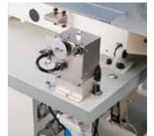
Constant-quantity bobbin thread feeding mechanism
