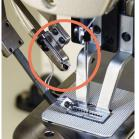
It holds the needle thread after thread trimming and prevents the needle thread from getting caught on the back side of the fabric.
