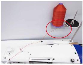
Put the thread inside the cone from the top, pass it through to the bottom, and use it by pulling it out from the thread groove of the base plate. The thread can be stabilized by passing through
