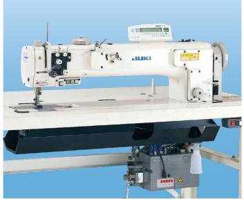
Long-arm, Unison-feed, Lockstitch Machine with Vertical-axis Large Hook
