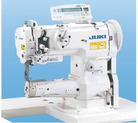
Cylinder-bed, 1-needle, Unison-feed, **Lockstitch Machine with Vertical-axis Hook**
