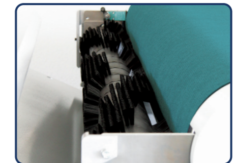
Cleaning brush: This optionally available cleaning unit eliminates any cutting residues
