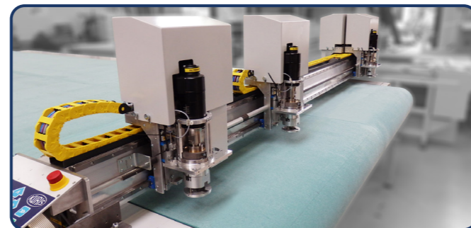
Cutting bridge with 4 cutting heads (cutter for carpet tiles)
